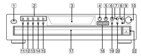
CHECK 20 (11, 12) CLEAR 9 (11, 12) DISC 1-5 **2** (8, 9, 11) Disc compartment [17] (7) DISC SKIP **8** (7, 10, 12) Display (9) EX-CHANGE 7 (10, 13) FADER 13 (12) PEAK SEARCH [12] (13)
